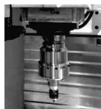
Ultrasound spindle to cut honeycomb plate (opt.)
